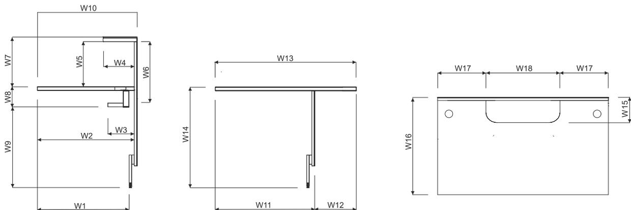
W1 - 763mm | W2 - 800mm | W3 - 200mm | W4 - 228mm | W5 - 329mm | W6 - 424mm | W7 - 365mm | W8 - 151mm | W9 - 589mm | W10 - 822mm | W11 - 822mm | W12 - 300mm | W13 - 1122mm | W14 - 740mm | W15 - 200mm | W16 - 800mm | W17 340/540mm | W18 - 520mm
